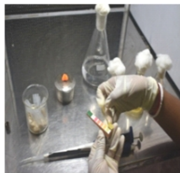
FIG A: the reagents were autoclaved; FIG B: after autoclaving the solutions were kept inside the laminated for cooling ; FIG C: the pH of the solutions were tested by using parchment paper
